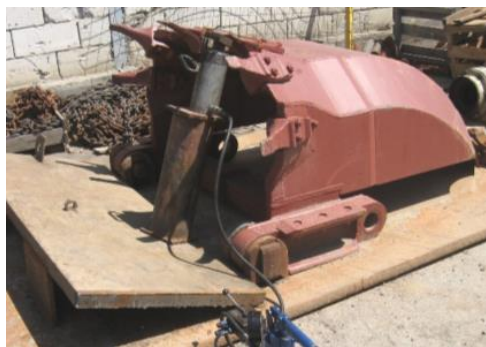
Figure 3. Laboratory testing for maximum bucket tooth load and virtual prototype.
